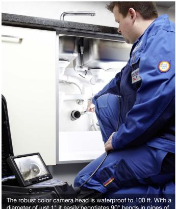
diameter of just 1" it easily negotiates 90° bends in pipes of 1 1/2" dia and larger.
