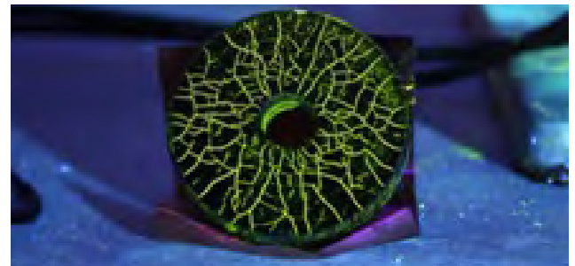
Example of 410HF/14HF fluorescent indications on an ISO 9934 Type 1 reference block.
