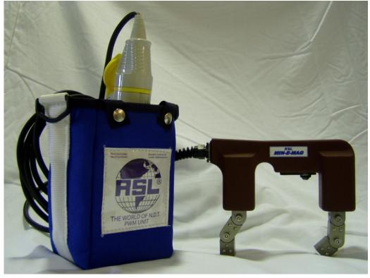
The PWM (Pulse Width Modulation) is a portable DC battery operated power supply that energises most makes of Electromagnets. The unit has two power settings High and Low. At the High setting it will lift the 18Kg test weight.
