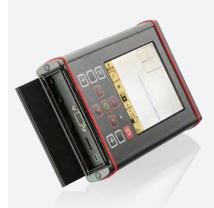
Under the flap there is a USB Connection for fast data transfer, SD Card Slot and VGA output for classroom and head-up display use.
